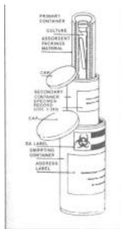
Fig.1.1: Diagram illustrate packaging and labeling of etiologic agents in volumes of less than 50 ml.
